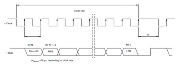
The following sketch and tabel illustrate possible malfunctions. For example, it is possible to analyse overtravel and under-run of the measurement range as well as an increasing distance between floating curser and transducer. This status is shown by the Alarm-Bit (Bit N).
